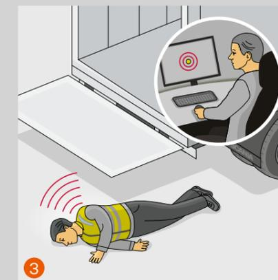
If the driver falls while outside the truck and becomes inactive, the Scania C-me’s sensor will trigger a call for help, while also relaying the GPS position. Using the connected app the driver can also actively send a text alert to a pre-set emergency number.
