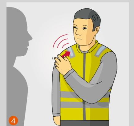
If the driver is exposed to a dangerous situation and the phone is inside the cab, the driver can still send an emergency alert by pressing five times on the vest.
